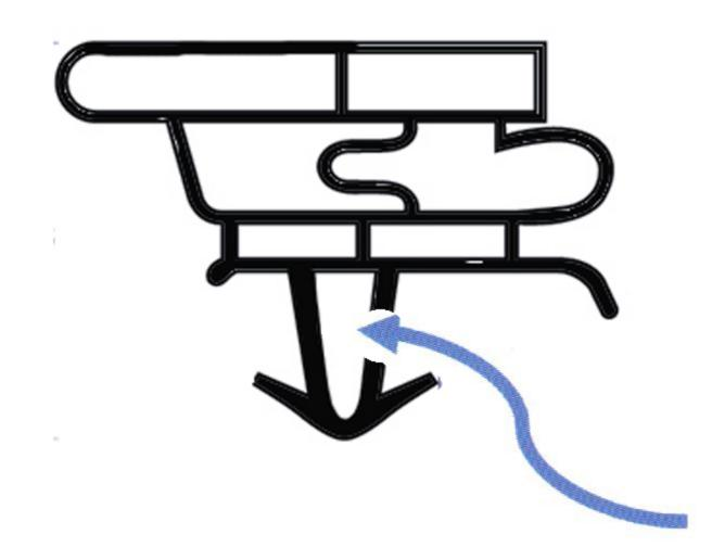
Arrow head that presses into slot around door
